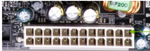
PWR1 connector Plug power cable from system power supply to PWR1
