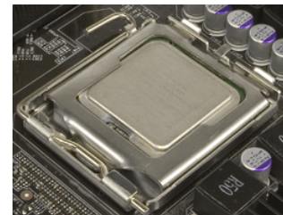
Align notches with notches on the CPU
